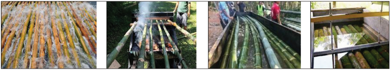
Figure 31: Bamboo Traditional Methods (Water Leaching, Smoking & Heating, Salt water immersion); (Bamboo U, 2024)
